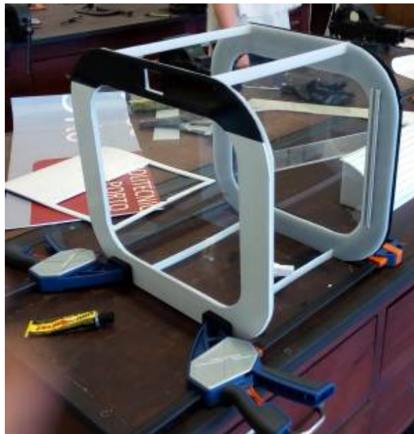
Figure 66: Assembly of the PVC walls with PMMA windows (53)
