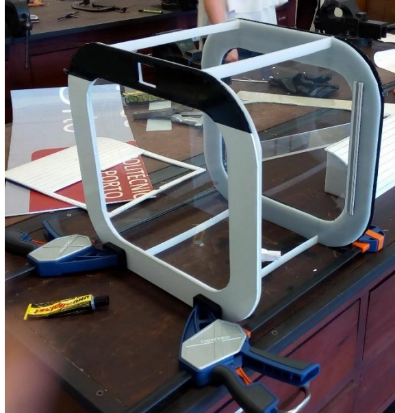
Figure 61 - Assembly of the PVC walls with PMMA windows (48)
